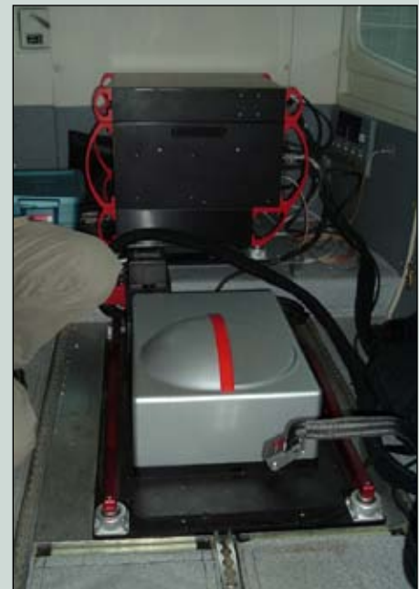
Figure 4—The Cessna Caravan and Leica ALS50 Phase 2 instrument that were used in lidar acquisition.
