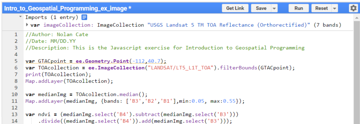
Figure 8: A screenshot of your script at this stage of the exercise showing ndvi being calculated
