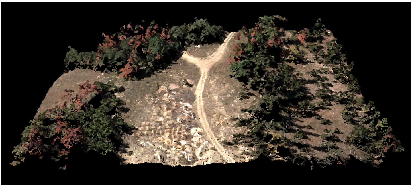
Figure 2 —A 3-D point cloud of an access road and trees located in Medicine Bow National Forest—derived from metric imagery processed with Imagine Photogrammetry.
