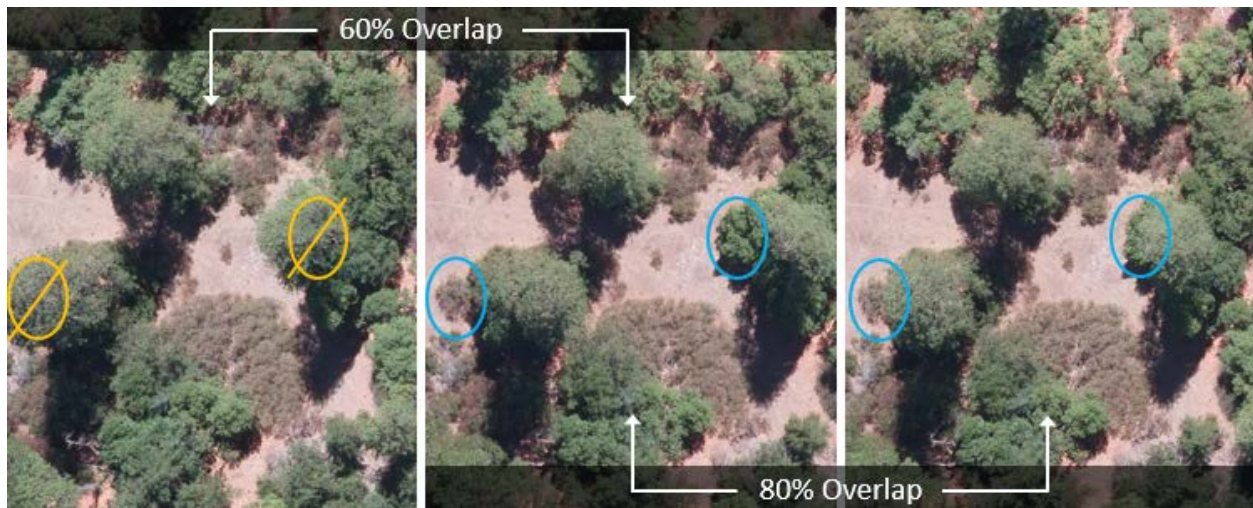
Figure 2: Some of the lower vegetation cannot be seen in both images with the 60% overlap (left and center). With 80% overlap, the circled vegetation can be seen and heights can be derived using phodar (bottom).
