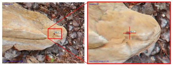
2. Markers can be placed on the individual images or directly on the mesh. Placing them on the mesh is helpful because Metashape will automatically place them on all images that the point intersects. To place the marker, make sure that the textured mesh is displayed in the main viewer and use your system mouse to zoom into the location of the first marker. Right click on
