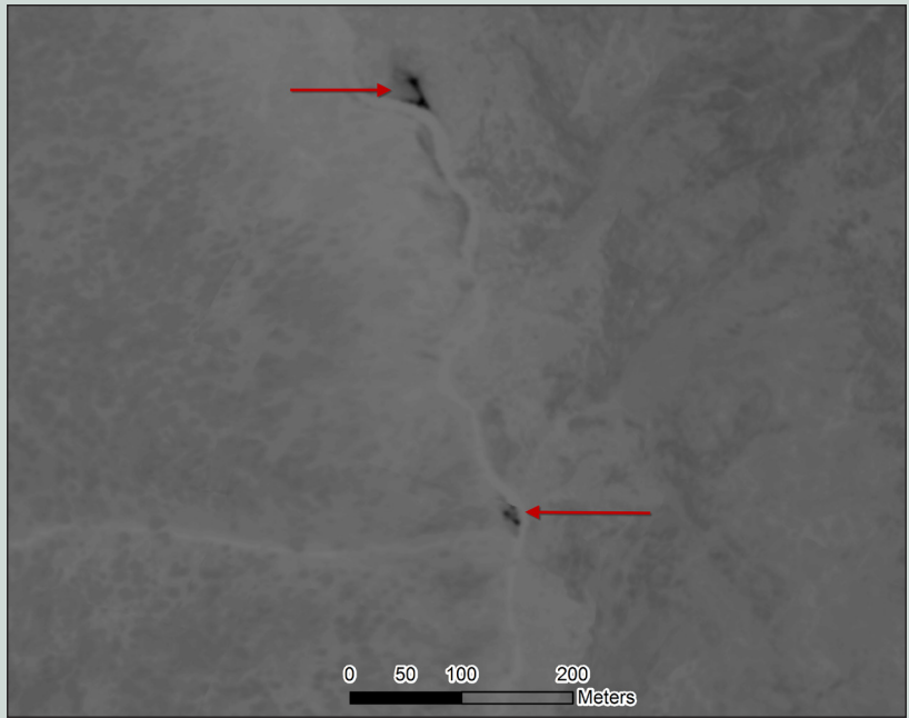
Figure 9—WAI LWIR imagery acquired on July 24, 2013 showing two apparent heat sources near the Ridge Fire that did not exceed the MWIR/LWIR ratio algorithm threshold. Further investigation revealed that the upper source was a gravel bar adjacent to the stream and the lower one was a hot spring in the stream channel.
