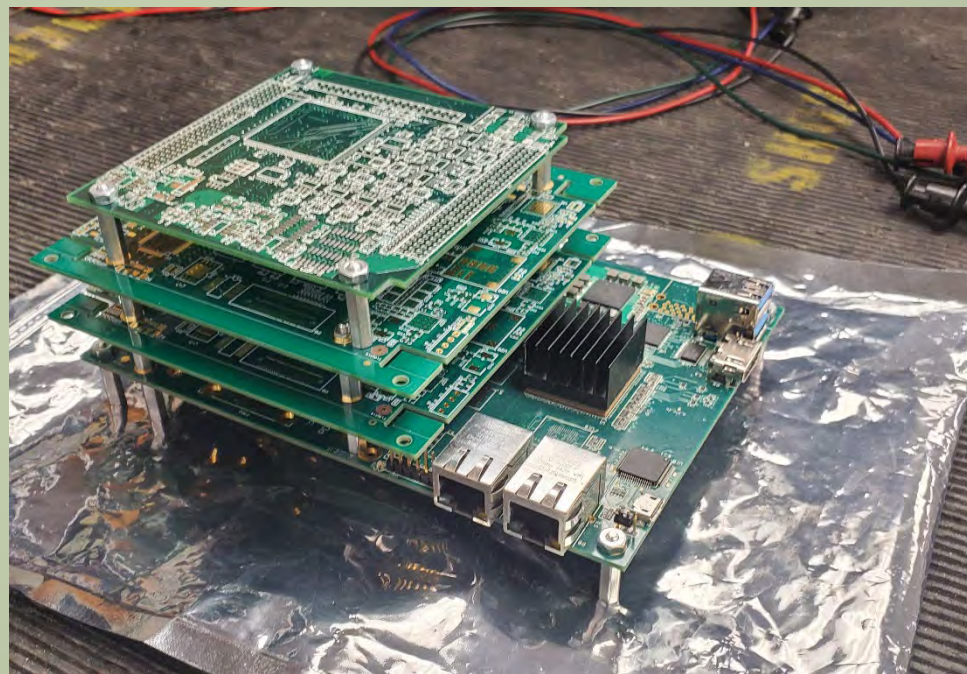
Figure 7: Single board computer with stacked ADC and DSP
