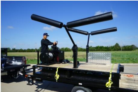
**The Mooring Platform** ~6' x 12', Turnkey operating base with power, helium, tools, winches; moved by forklift or helicopter; enables aerostat towing & two person operations; folds to fit ISO-20 container
