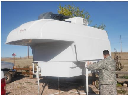
**Mobile Command Center** - Truck transportable, self-contained dual power, data storage, network control climate controlled work space. Auto-acquire SATCOM tracking and 50 MBps bandwidth. Input-Output ports for extended local communications
