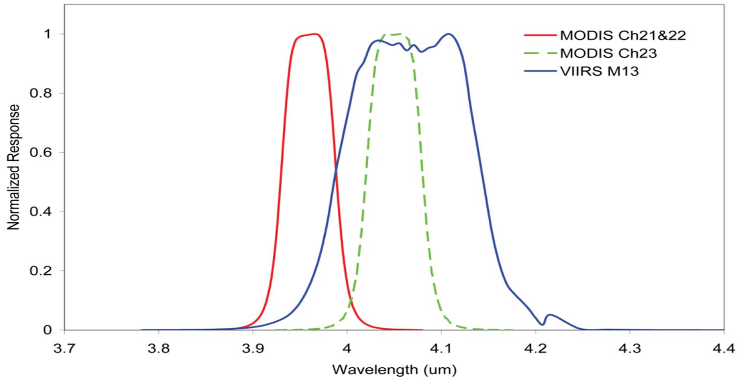
*Spectral response curves for MODIS channels 21-23, and VIIRS channel M13*
