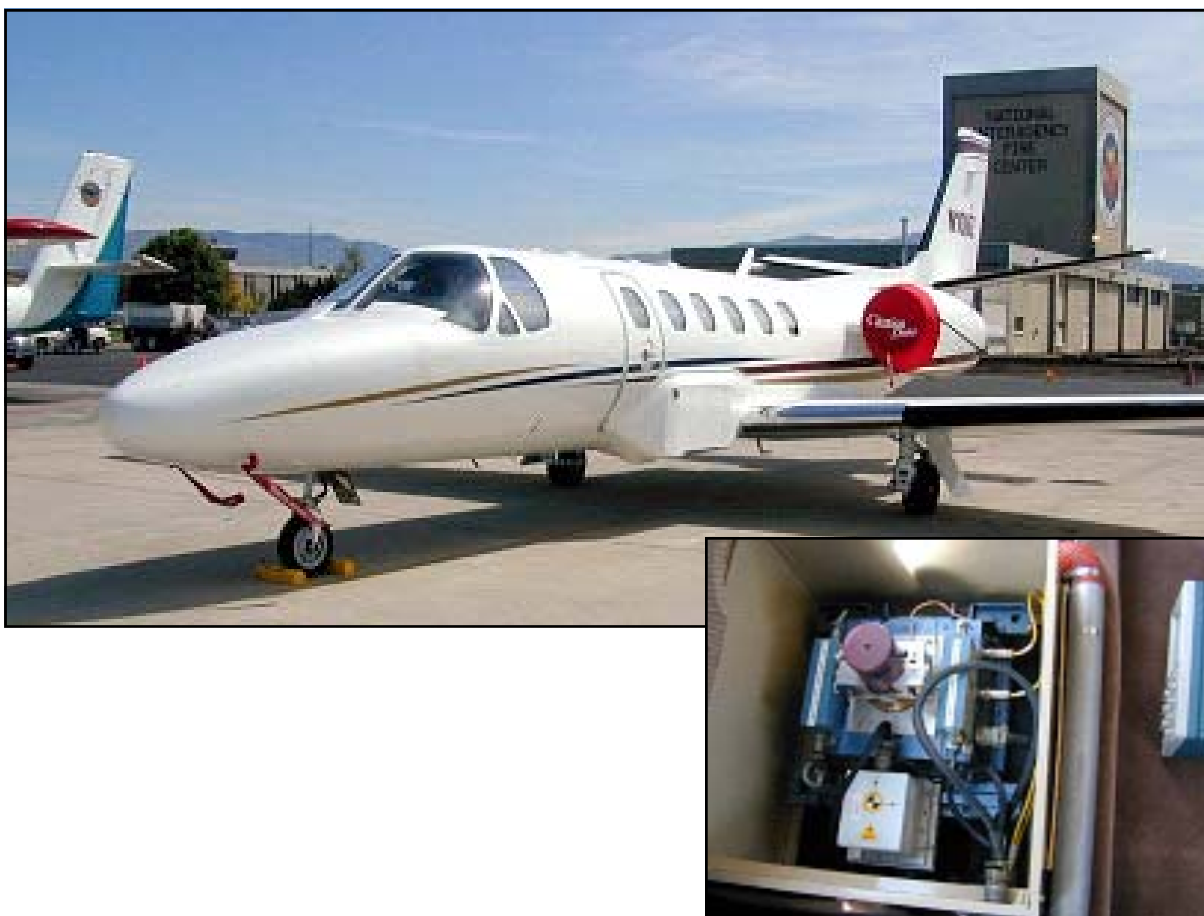
Figure 7—The NIFC Citation Bravo and the Phoenix line scanner, type 1 platform and sensor.
