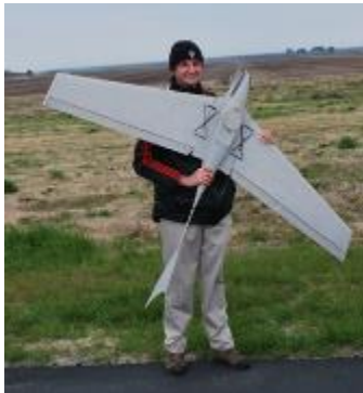
Super Swiper (Bosh Technologies) [9 lbs, 6ft wingspan]
