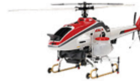
RMAX (Yamaha) [100 lbs, 10ft rotorspan]
