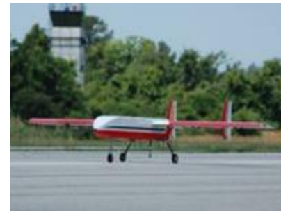
FENRIR (NCSU ARC Team) [45 lbs, 10 ft wingspan]
