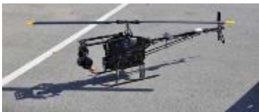
Condor II (Bosh Technologies / Leptron) [10 lbs, 6ft rotorspan]
