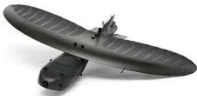
Maveric (Prioria Robotics) [3 lbs, 3ft wingspan]
