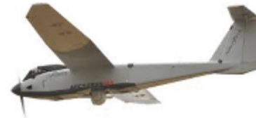
T-20 (Arcturus) [120 lbs, 20ft wingspan]
