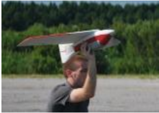
Vireo (FourthWing Inc) [3 lbs, 2.5 ft wingspan]
